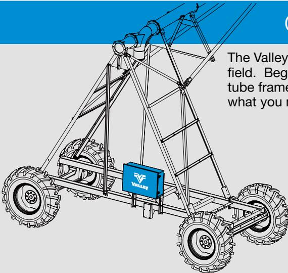
The Valley Rainger gives you the ability to customize the equipment to fit your field. Begin with the Valley linear basic cart, equipped with the durable five-inch tube frame. The same frame is used no matter your water source – you select what you need.
